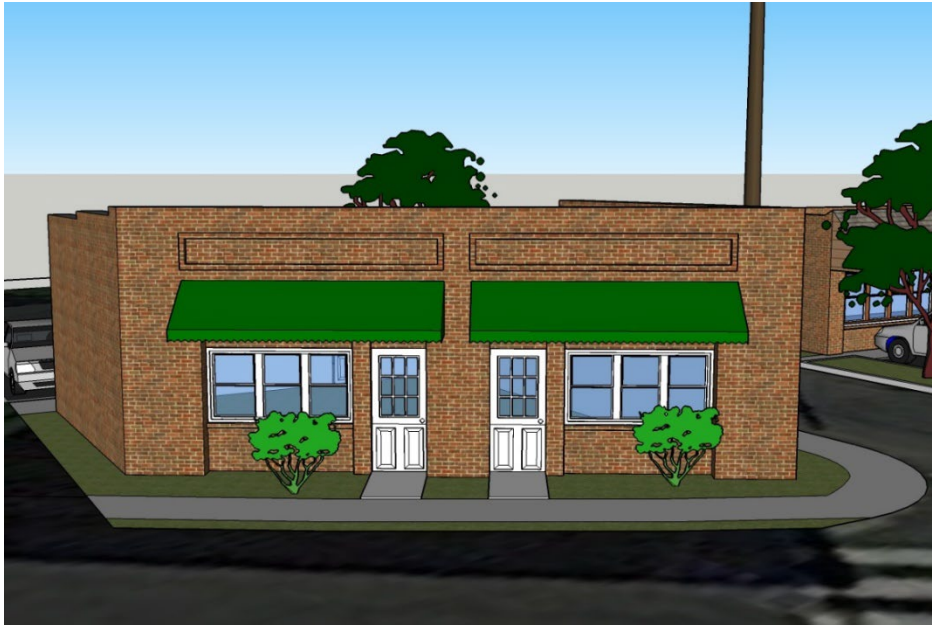
Remove window unit AC; clean and restore 3-bay window sets
